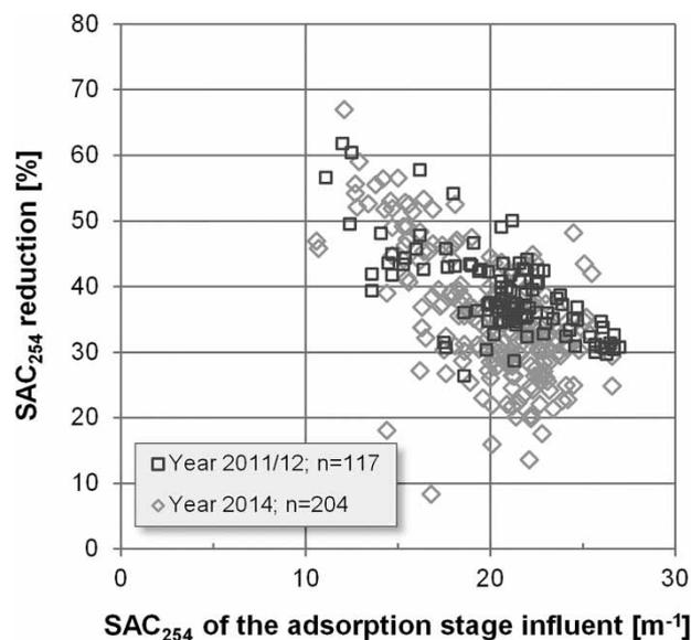
**Figure 3** | SAC<sub>254</sub> reduction versus the SAC<sub>254</sub> of the adsorption stage influent at a dosage of 10 mg PAC/L.
