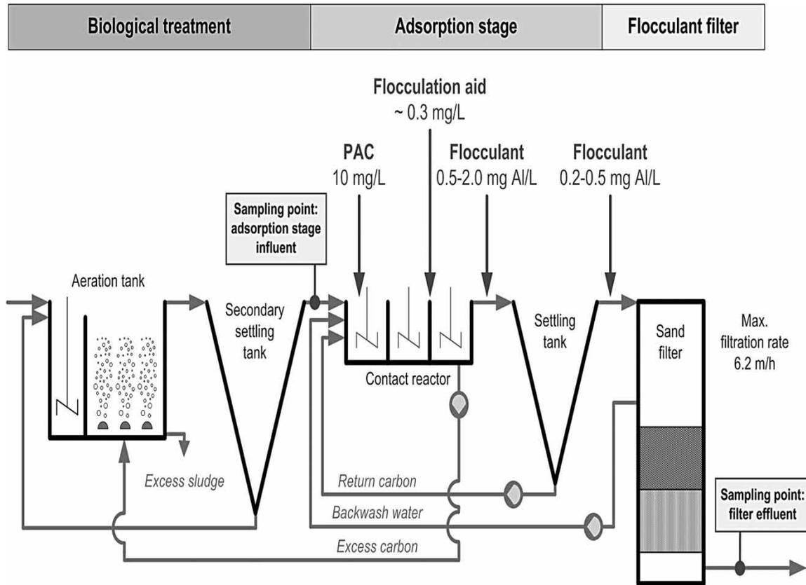
**Figure 1** | Process diagram of the OMP adsorption stage at the Mannheim WWTP.
