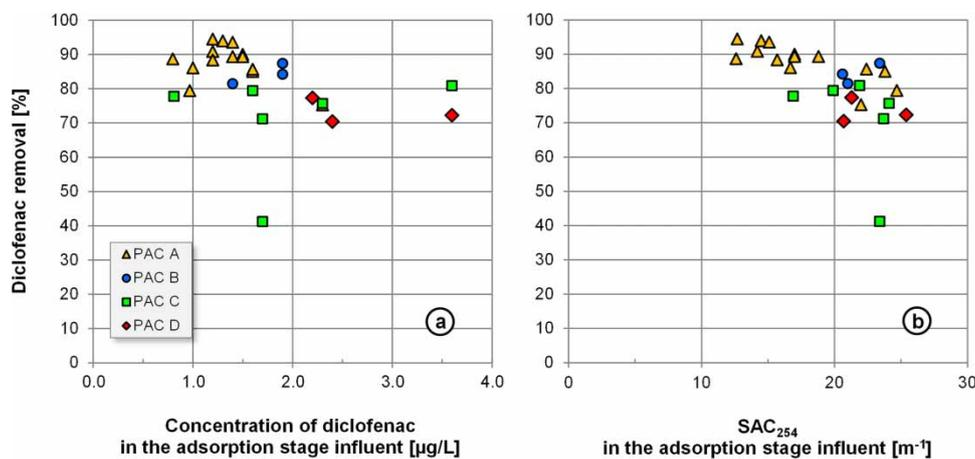
**Figure 4** | Diclofenac removal at a dosage of 10 mg PAC/L varying with the concentration of diclofenac in the adsorption stage influent (a) and with the SAC<sub>254</sub> of the adsorption stage influent (b).
